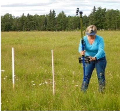
Collected grass samples in pasture fields. Each sample has a corresponding “vegetation index value” acquired with a handheld spectrometer calibrated to the satellite.
